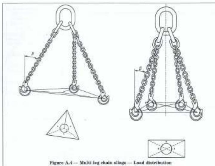
Figure A.4 — Multi-leg chain slings — Load distribution
