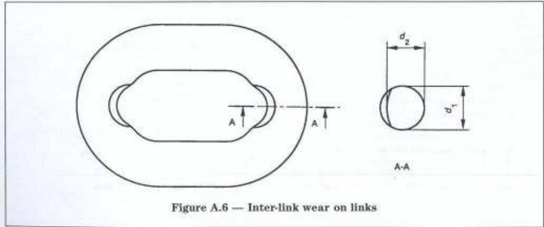
Figure A.6 — Inter-link wear on links
